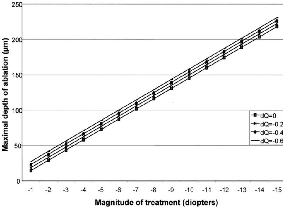
FIGURE 5. The influence of the variation of asphericity on the maximal depth of ablation. For the same magnitude of myopia treatment, the maximal depth of ablation increases when  $dQ$  is negative (increased prolateness of the final corneal profile). This additional depth is proportional to the absolute value of  $dQ$  and is independent of the initial asphericity or the magnitude of dioptric correction.
