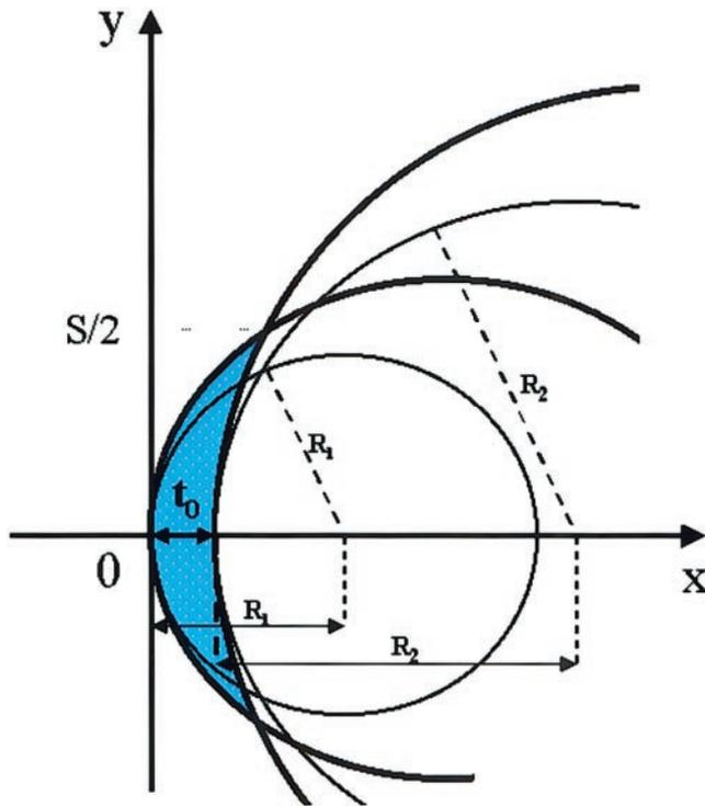
**FIGURE 1.** The aspheric profile of ablation (*blue zone*) corresponds to the difference in sagittal height between the initial and final corneal surfaces on an optical zone of diameter  $S$ . The initial and final corneal profiles are aspheric and modeled as conic sections of apical radii  $R_1$  and  $R_2$ , and asphericities of  $Q_1$  and  $Q_2$ , respectively. The maximal depth of ablation ( $t_0$ ) occurs at the center of the optical zone.
